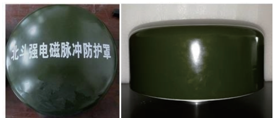
Fig. 7 Strong electromagnetic pulse protective radome for Beidou navigation receiver
