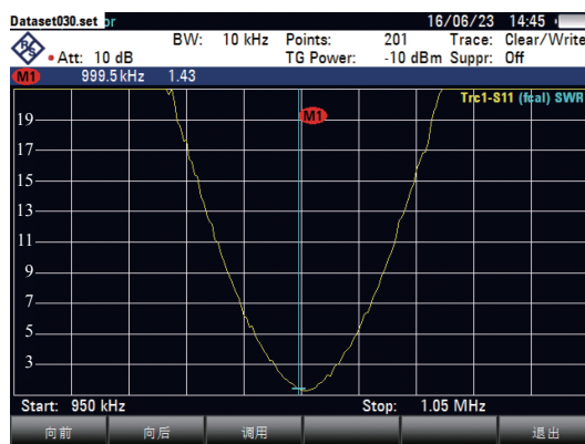
Fig. 7 Measured value of vector network analyzer
