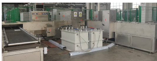
Fig. 1 Radiation device for sterilization of the packing box surface
