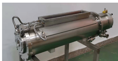
Fig. 2 Main part of electron curtain accelerator
