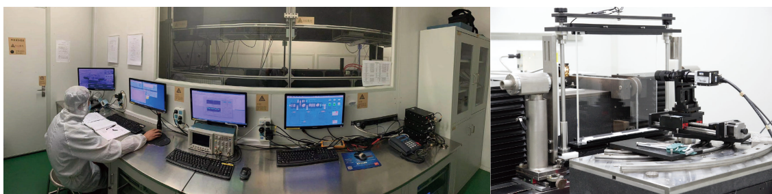
Fig. 13 Laser conditioning platforms for large size DKDP crystals [89]
