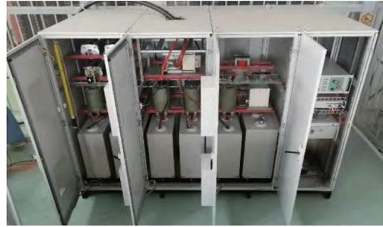
Fig. 11 Pulse power supply device
