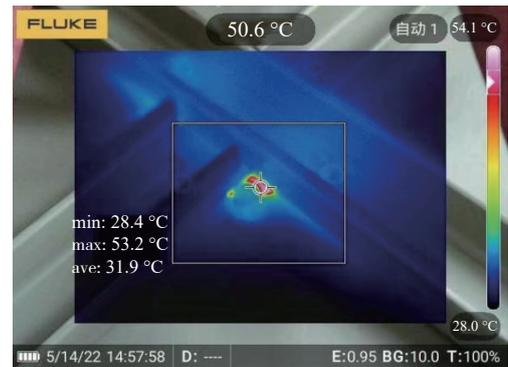
Fig. 13 Maximum temperature position of pulse inductor temperature rise experiment
