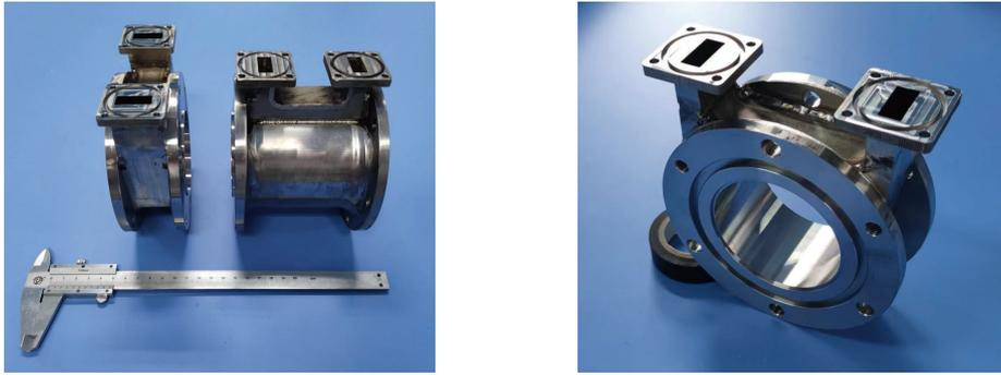
Fig. 7 Photos of double hole directional coupler
