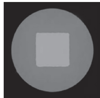
Fig. 16 Cross section of a rectangular core fiber
