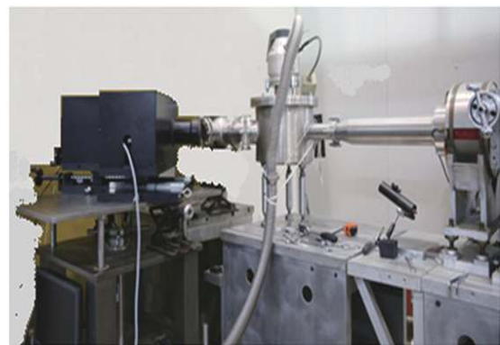
Fig. 3 Beam divergence measurement system and layout
