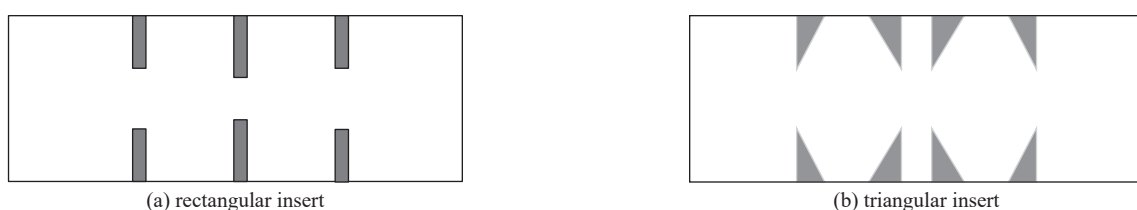
Fig. 1 Comparison of conventional filter with rectangular insert and novel filter with triangular insert
