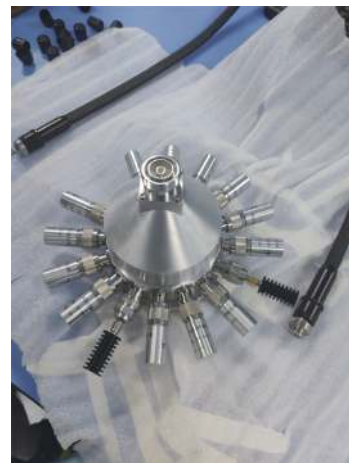
Fig. 6 Machined power divider
