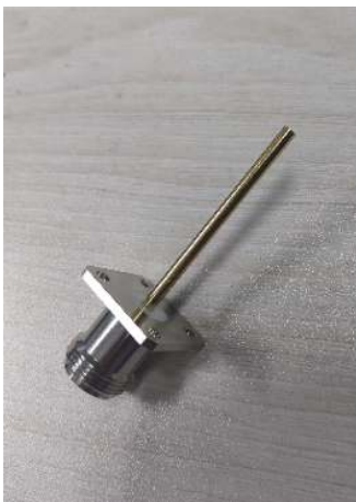
Fig. 5 Designed N-type connector
