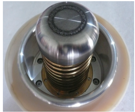
Fig. 9 Internal photo of the pulse compression device after outputting 300 000 pulses
