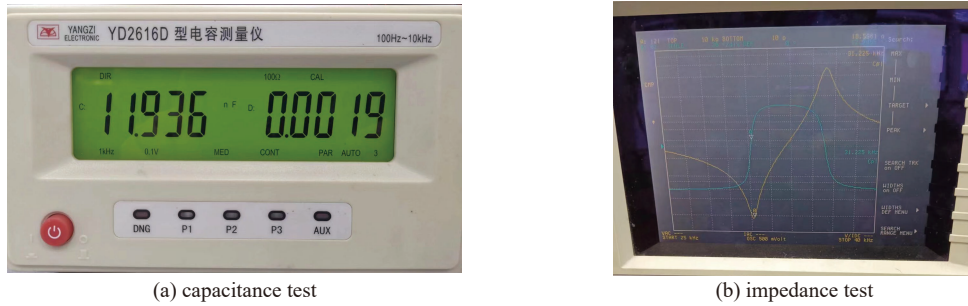
Fig. 2 Capacitance and impedance curve of piezoelectric ceramics
