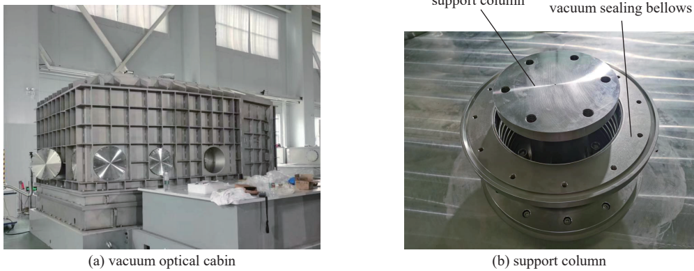
Fig. 9 Vacuum optical cabin without negative pressure
