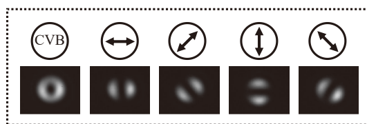
Fig. 4 Beam intensity distribution before and after passing through a rotatable polarizer
