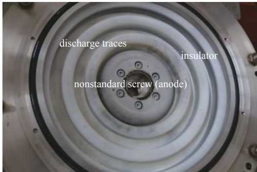
Fig. 1 Insulator and nonstandard screw (anode)
