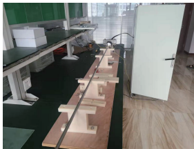
Fig. 7 Electromagnetic loading Hopkinson bar experiment
