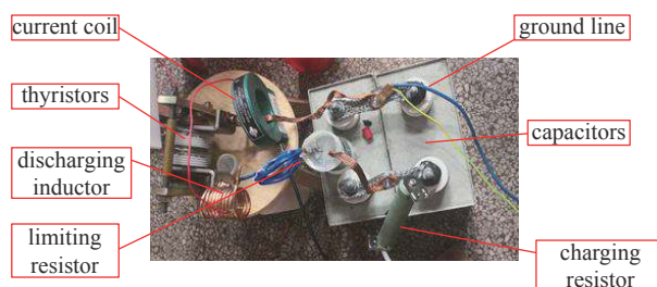
Fig. 5 Experimental test of thyristor temperature rise
