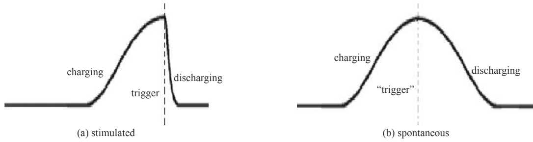
Fig. 5 Typical discharging waveforms in LIA pulsed power system
