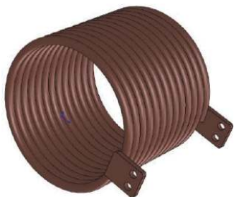
Fig. 4 Diagram of repetitive frequency water-cooled inductor coil
