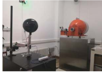
Fig. 6 Experimental device for measuring radioactive sources in a 10L spherical ionization chamber
