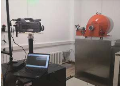
Fig. 5 Experimental device for measuring radioactive source with high purity germanium detector
