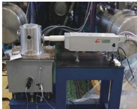
Fig. 5 Picture of the trigger unit and No.0-laser
