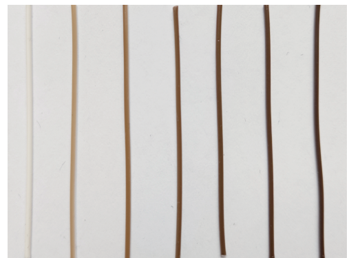
Fig. 2 VUV radiation time on appearance color of X-ETFE cable 图 2 VUV 辐照时间对外观颜色的影响
