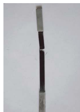
Fig. 3 Damage outlines of CFRC laminate after mechanical tensile test
