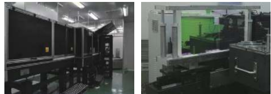
Fig. 14 Laser conditioning platforms for large optics [35]
