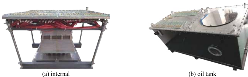
Fig. 7 Photos of pulse transformer
