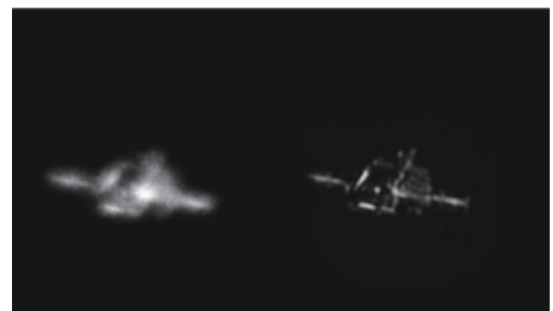
Fig. 10 Daytime observation of the International Space Station: (left) unreconstructed image; (right) PD reconstructed image
