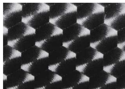
Fig. 4 Microlens arrays for microlens array scanners made in the Lincoln Laboratory at MIT using binary optics
