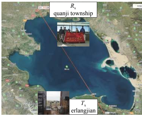
Fig. 1 Diagram of 100 km of Xi'an University of Technology wireless optical communication experimental link
