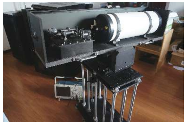
Fig. 2 Photo of internal structure of wireless coherent optical communication
