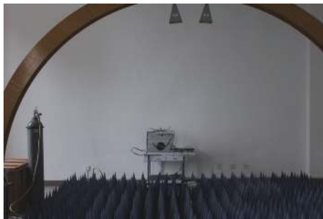
(a) microwave reflection arch test
