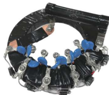
Fig. 4 Photograph of the produced five-stage LC-Marx generator
