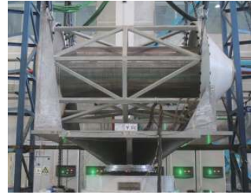
Fig. 12 Vibration test of PFL equivalent parts 图 12 形成线等效件振动试验
