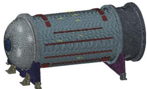
Fig. 8 Finite element model of PFL under clamped boundary condition
