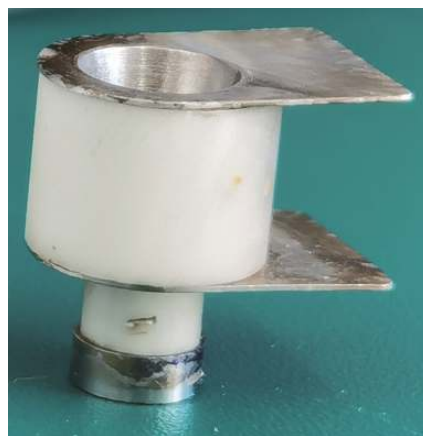
Fig. 2 Sample of gas-breathing triggered vacuum switch
