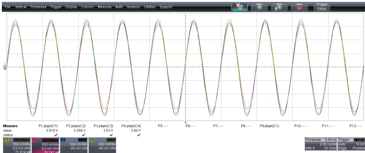
Fig. 10 Amplitude-phase consistency testing of BPM RF front-end electronics module
