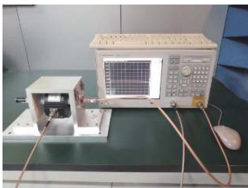
Fig. 3 Vector network analyzer test device
