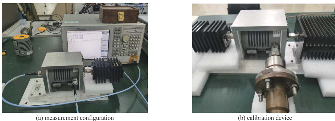
Fig. 12 Physical configuration of current injection probe performance test
