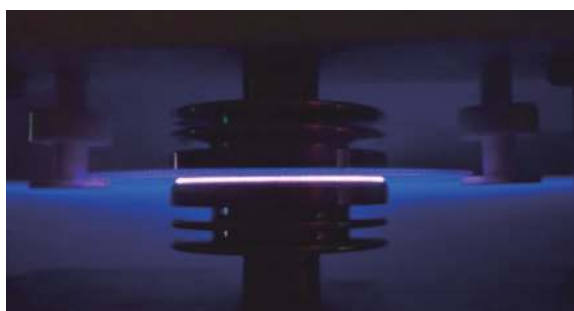
Fig. 12 Photo of DBD excited by the High voltage pulses from the Marx generator
