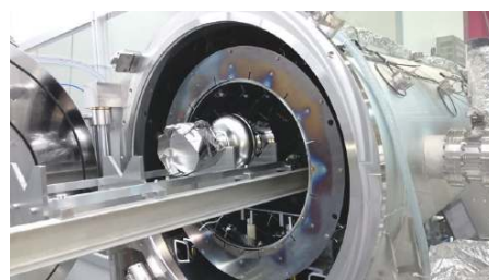
Fig. 6 N-doping of 1.3 GHz cavity
