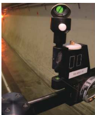
Fig. 2 Optical-wire position system/sensor
