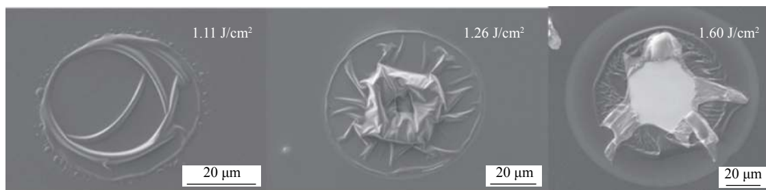
Fig. 3 Typical damage morphologies of the PI/ITO/glass sample
