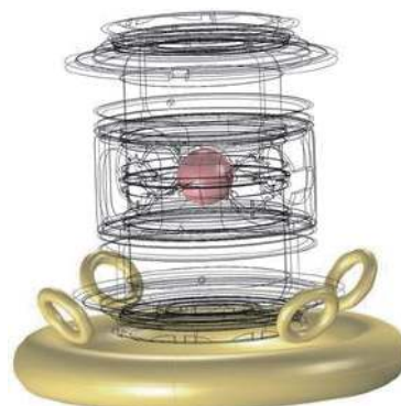
Fig. 11 Schematics of the superconducting magnetic levitation to support capsule
