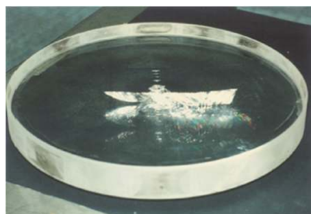
Fig. 1 Damage and crack of fused silica optics caused by transverse stimulated Raman scattering (TSBS) effect
