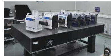
Fig. 8 Partially commercialized streak cameras developed in XIOPM 图 8 是部分商业化条纹相机实物照
