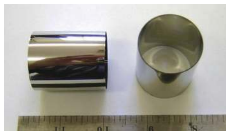
Fig. 6 Picture of Wolter microscope objective applied to Z-pinch device
