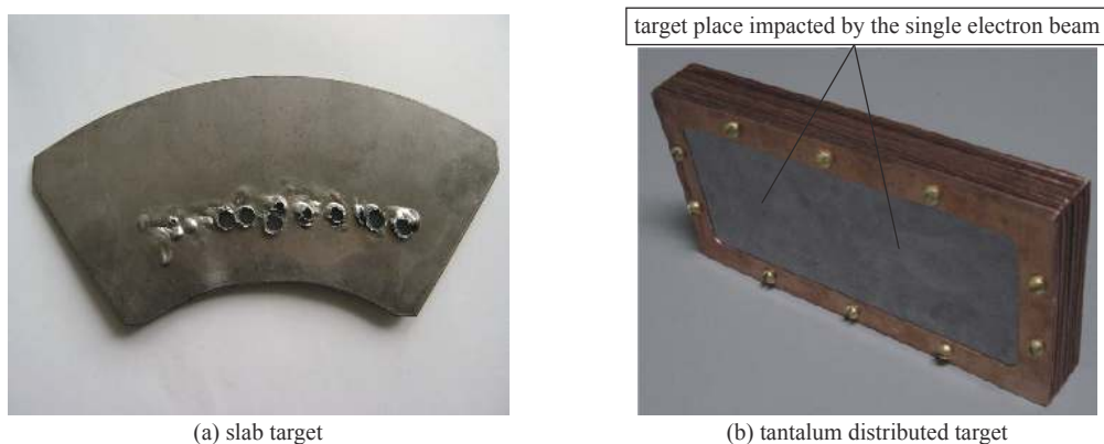
Fig. 4 Damage of different targets for 12 MeV LIA
