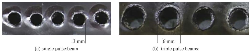
Fig. 6 Damage of the tantalum distributed target impinged by different electron beams from Dragon- II accelerator
