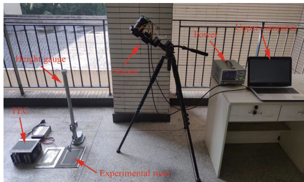
图3 实验系统图 Fig.3 Experimental system diagram
