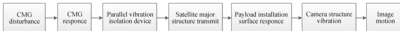
图11 高分多模卫星微振动对成像质量影响链路 Fig.11 GFDM-1 satellite impact link of micro-vibration to imaging quality
