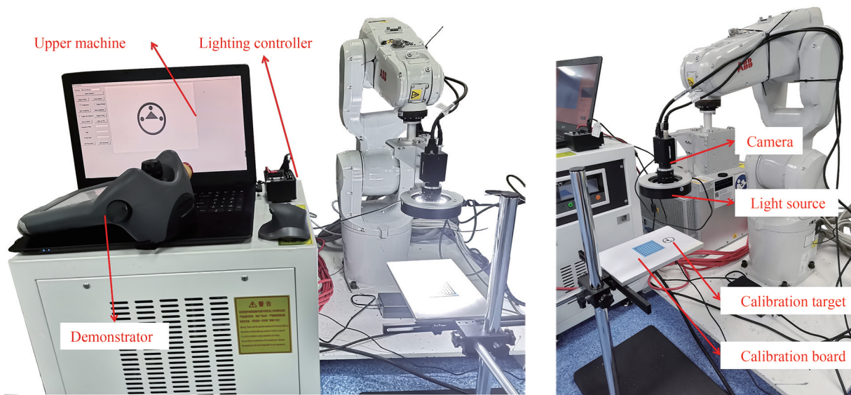
图8 空间平面位姿测量实验平台 Fig.8 Experimental platform of spatial plane pose measurement
