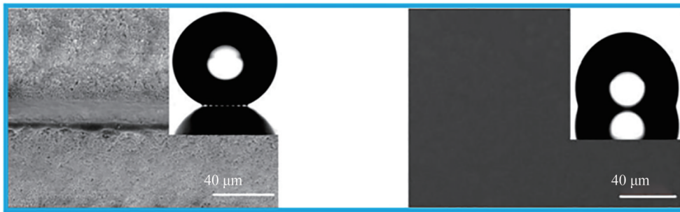
(a) The morphology and contact angle of the K9 glass surface ablated by femtosecond laser and the smooth K9 glass surface
