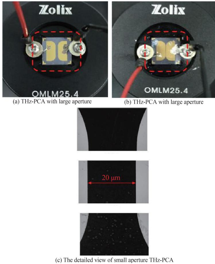
Fig. 20 The view of home-made THz-PCAs
