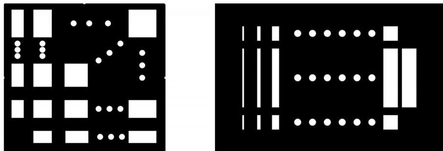
(a) Mask plate corresponding to doping distribution in Fig. 3 (b) Mask plate used in pixel design in this section
