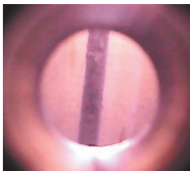
图6 压力80 Pa微波800 W时同轴线型CH 4 等离子体 Fig. 6 Coaxial line CH 4 plasma driven by 800 W microwave at fill pressure of 80 Pa
